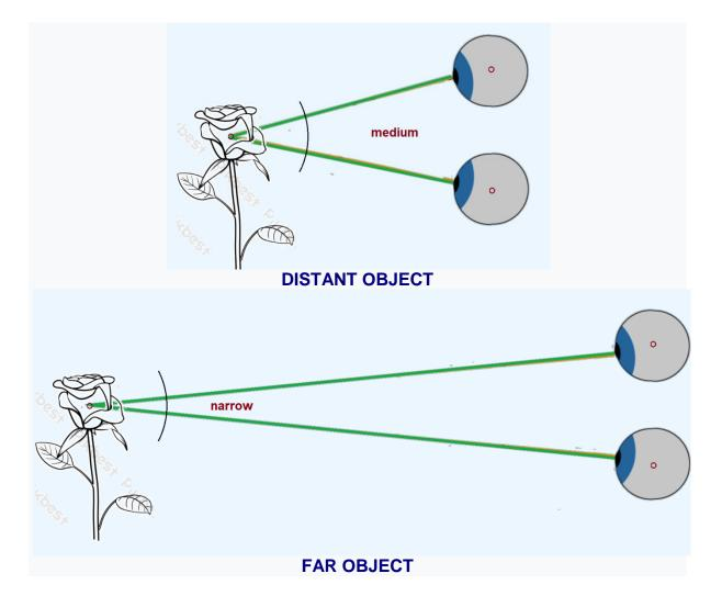
As we see, in real life the visual axes angles reduces as object goes far, but, -All commercial adapters including the costly ones, operate exactly at the REVERSE way they would do. -
