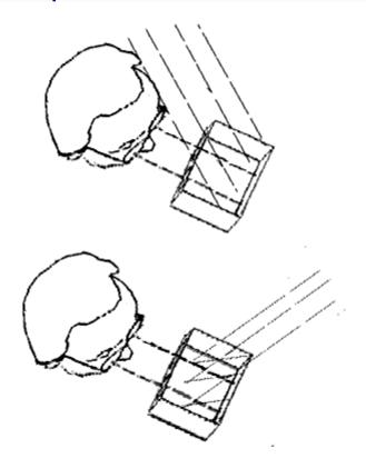
Fig 5 Two favorable image lighting conditions on the SSV-2.
