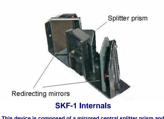
This device is composed of a mirrored central splitter prism and two redirecting external mirrors.
