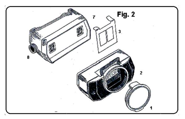
Mounting the device for slide viewing
