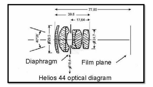
Helios 44 optical diagram and real dimensions.
